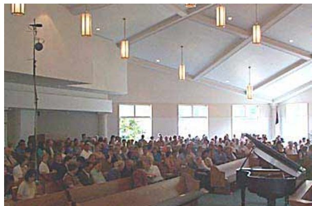
Fig.9 - shows the PerAmbio 6.1.10+main microphone array in a recital hall for experimental recordings to test dual format 2D/3D. Mode j' ("juxtaposed", high and tilted) was preferred for ITU6.1 transformation.
