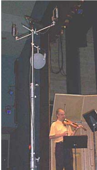
Fig.2 PerAmbio 6.1.10+ test microphone array in the concert hall.
