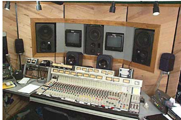
Fig.11 - Multi-format control room monitoring (showing 7 of 18 speakers +2 subwoofers) is switchable between PerAmbio 6.1.10 and ITU 5.1/6.1 (no need to change listening position as in Fig.1). The common “Sweet spot” accommodates two within the control room’s reflection free zone (RFZ). In addition to Periphonic 3D surround demonstrations, this facility produces compatible 5.1 and PanAmbio 4.1 mixes, including evaluation CDs available to audio engineers at www.filmaker.com .
