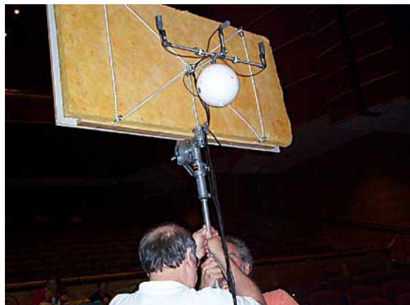
Fig. 15. Hoisting OCT and prototype Ambiophone microphones in the 1,000 seat opera house. Microphones are Schoeps CCM-series.
