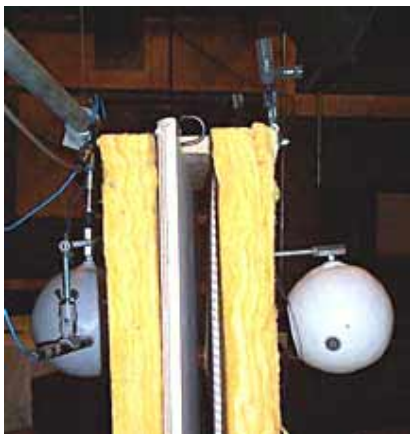
Fig. 14. OCT atop prototype "PanorAmbiophone" – twin sphere microphones separated by baffle. In the studio, the rear sphere also served as room microphone for OCT.
