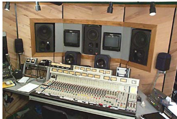
Fig.8 - Multi-format control room (7 of 19 speakers visible) for mixing stereo, 5.1, and HSD-3D (full sphere, with height).
