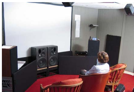
Fig.7 - Demonstration “home theater” (7 of 10 speakers visible) for replay of stereo, 5.1, and HSD-3D (full sphere, with height).
