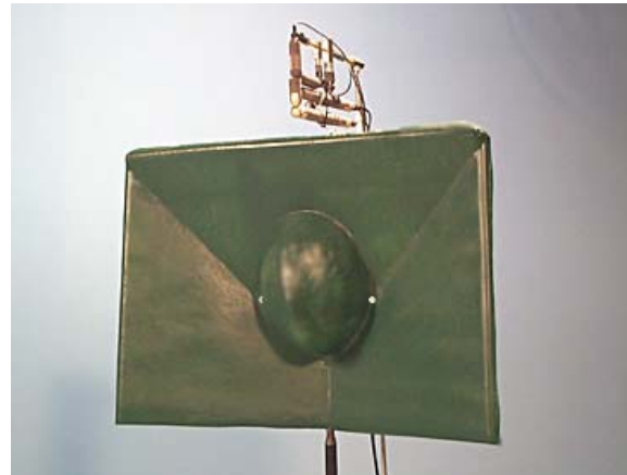
Fig.1 - HSD microphone showing front of baffled ellipsoid and discrete soundfield array mounted above (total 8 microphones).
