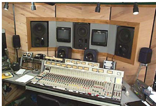
Fig.3 - Multi-format control room (7 of 19 speakers visible) for mixing stereo, 5.1/6.1, and HSD-3D (full sphere, with height).
