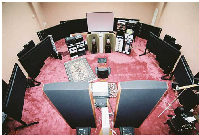
Pair #5 above are SoundLab Majestics , full-range electrostatic speakers (bi-directional) in the foreground, pictured at the Ambiophonics Institute, that compared very favorably to all five live sources in the experiment.
