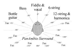
Fig. 3. PanAmbio 4.1 (2/2) reproduction localizes sources accurately within  $\pm 5^{\circ}$ , virtually duplicating the recording session directions in Fig. 5 below. Guitar quintet and fans are placed as shown for experiments that contrast two 360° reproduction methods. Multi-channel surround sound is more "realistic" by localizing both front stage instruments and sounds from around and behind, including antiphonal voices, audience participation, and ambience.
