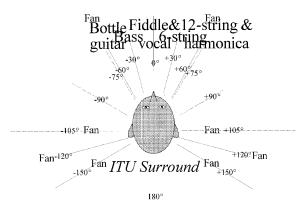
Fig. 4. Contrasted with PanAmbio, ITU 5.1 "relocates" quintet+fans by angular distortion (although less than two-speaker stereo). Original angles indicate sounds recorded at  $\pm 75^{\circ}$  are heard at  $\pm 30^{\circ}$  and are superimposed within the band. If precision localization is not essential to a recording, ITU 5.1 may be quite acceptable.
