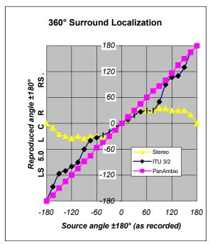
Fig. 7. Perceived localization around entire 360° horizontal plane – ITU 5.0 vs. PanAmbio 4.0. Listeners reported to the nearest 5° that ITU 5.1 (3/2) is "ambiguous" at  $\pm 90^{\circ}, \pm 105^{\circ}, \pm 120^{\circ}, and \pm 150^{\circ}$ . PanAmbio 4.0 approaches the ideal straight line but is "fuzzy" nearing  $\pm 90^{\circ}$ , coinciding with the "cone of confusion" of human hearing.
